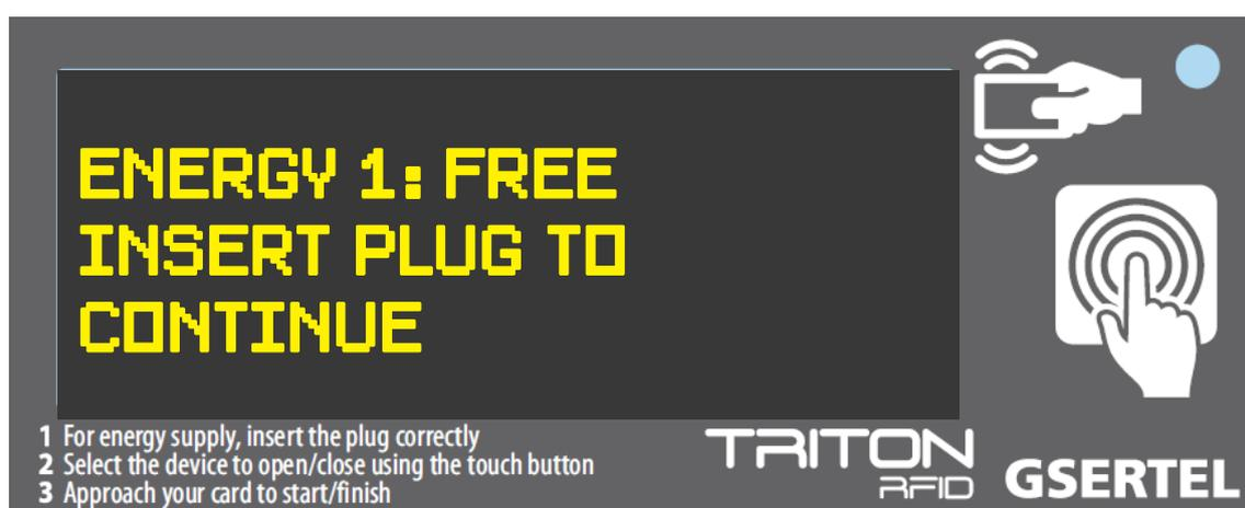
If the pedestal has the plug detector enabled, you must insert the plug correctly before you can open the socket. When the plug is detected correctly, the display will show this message:
